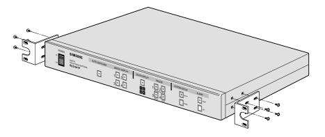
After you have attached both mounting adaptor to the SCQ-041P, align the SCQ-041P within the appropriate space in the rack and attach it firmly to the rack.
